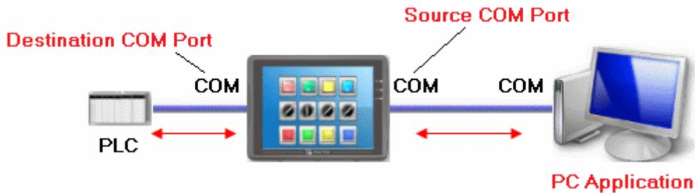
**Source COM Port:** This port is connected between HMI and PC.
