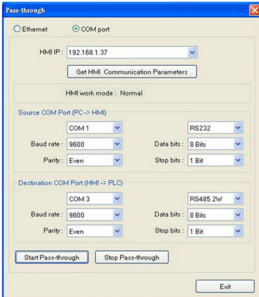
User can press [**Start Pass-through**] (the HMI work mode is switched to “ Pass-through”) and to run On-line Simulation. Now PC application can control PLC via HMI, and HMI is acting as a converter; meanwhile the HMI don't have function until stop pass-through.
