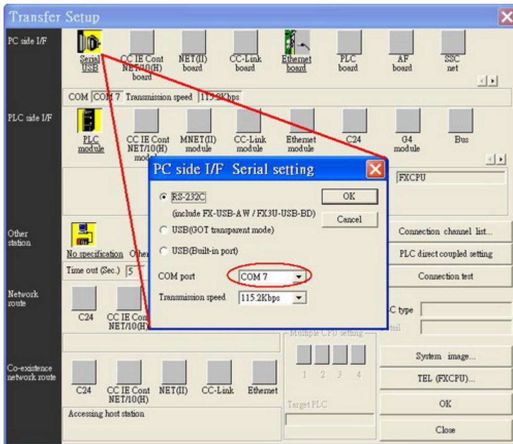
After completed all of described setting, when user running the PLC application on PC, the HMI will auto be switch to pass-through mode (the communication between HMI and PLC will be suspend). And it will resume communication if user closes the application, as follow
